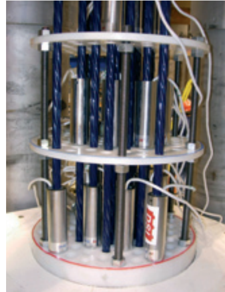
DYNA Force™ in Fatigue Test of Cable Stay System
